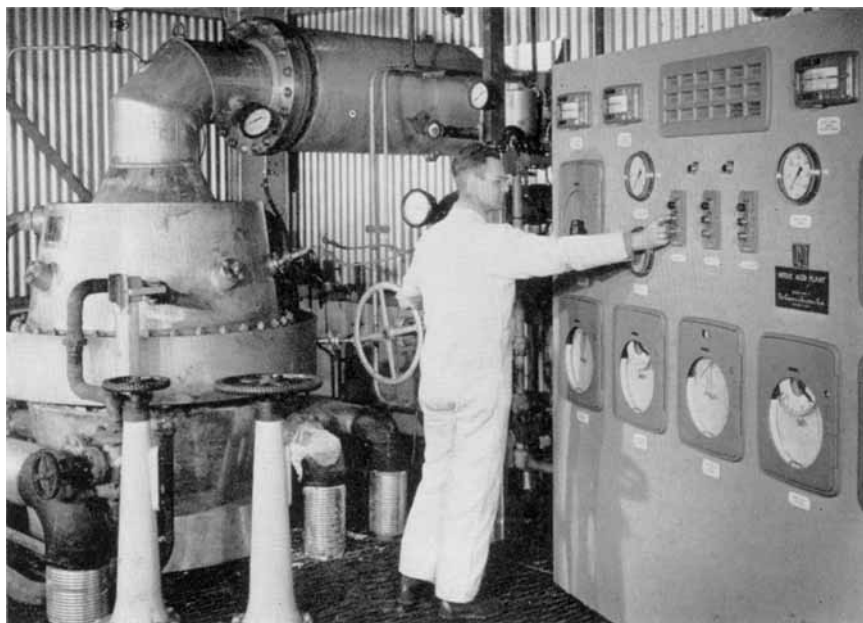
The converter and control panel. The converter contains the catalyst, consisting of a pack of 36 hexagonal gauzes woven from rhodium-platinum alloy wire
