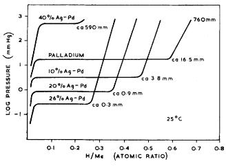
Fig. 7 Isotherms for Ag-Pd-H systems at  $25^{\circ}C$
