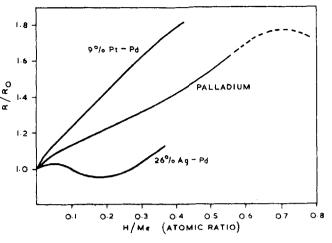
Fig. 5 Relationships between relative electrical resistance and hydrogen content
