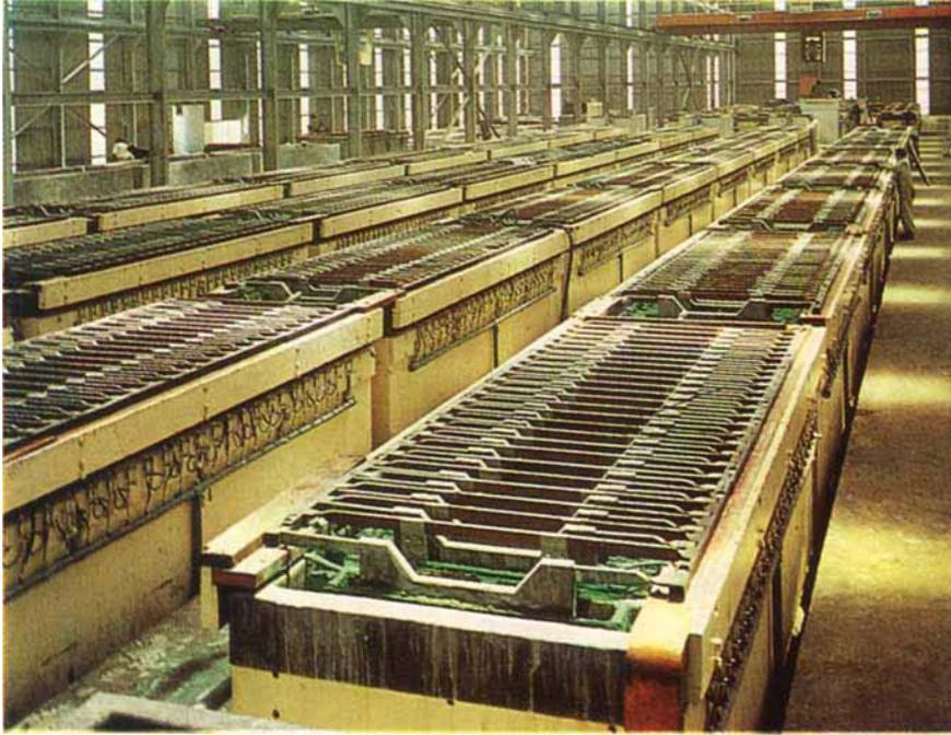
*In the electrolytic nickel refineries pure nickel cathodes are produced while the platinum metals accumulate in the anode residues and are removed for separation and refining*
