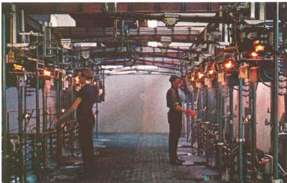
*The manufacture of glass fibre involves the rapid flow of glass at around 1,400°C through a series of orifices which must retain their size and alignment. The electrically heated bushings are universally made in rhodium-platinum alloys*
