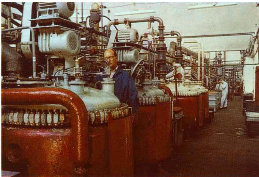
*The initial stage in the Johnson Matthey wet process refinery involves digestion of the enriched concentrates with aqua regia to dissolve the platinum and palladium, leaving the iridium, rhodium, ruthenium and osmium as insoluble residues to be treated separately*
