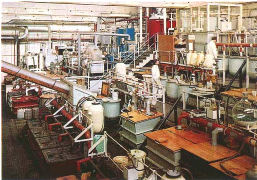
*This section of the Johnson Matthey refinery – the largest of its kind in the world – handles the precipitation, re-dissolving and re-precipitation of platinum and palladium*
