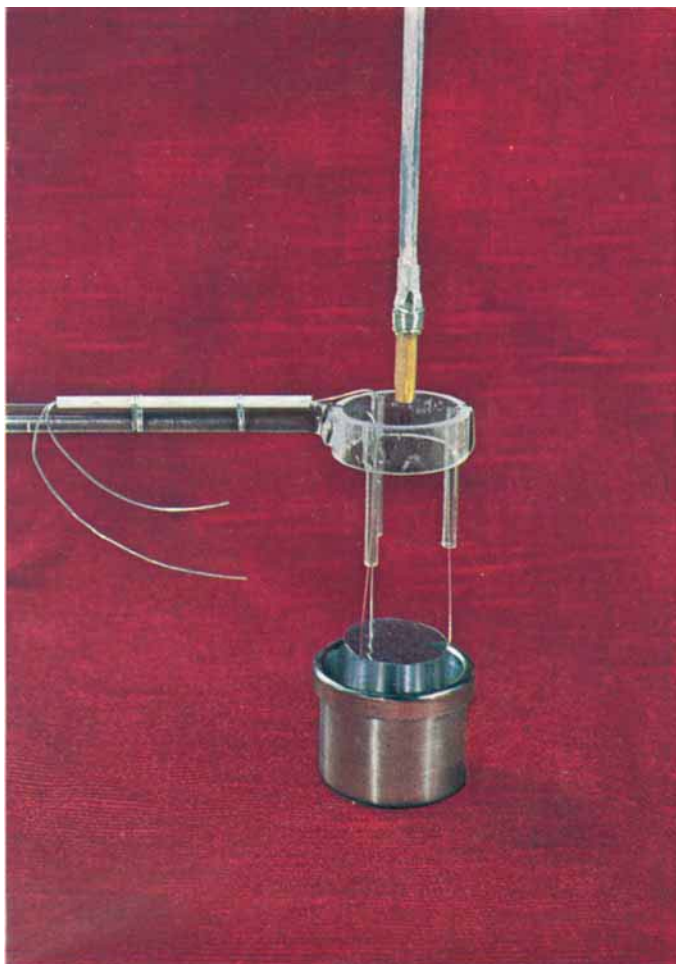
Fig. 2 Some platinum components used in crystal growth. At the top of the photograph is a seed holder, in the centre is a silica ring from which is suspended a platinum baffle for suppressing thermal oscillations, and at the bottom is a crucible with a reinforced rim
