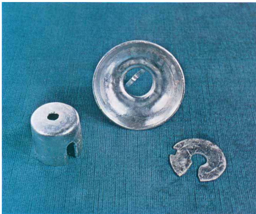
Fig. 3 Various heat shields to decrease the temperature gradient in growing crystals. The beehive shape is fabricated from iridium and the others from platinum. These shields couple to the radio frequency field and act as additional heat sources above the melt
