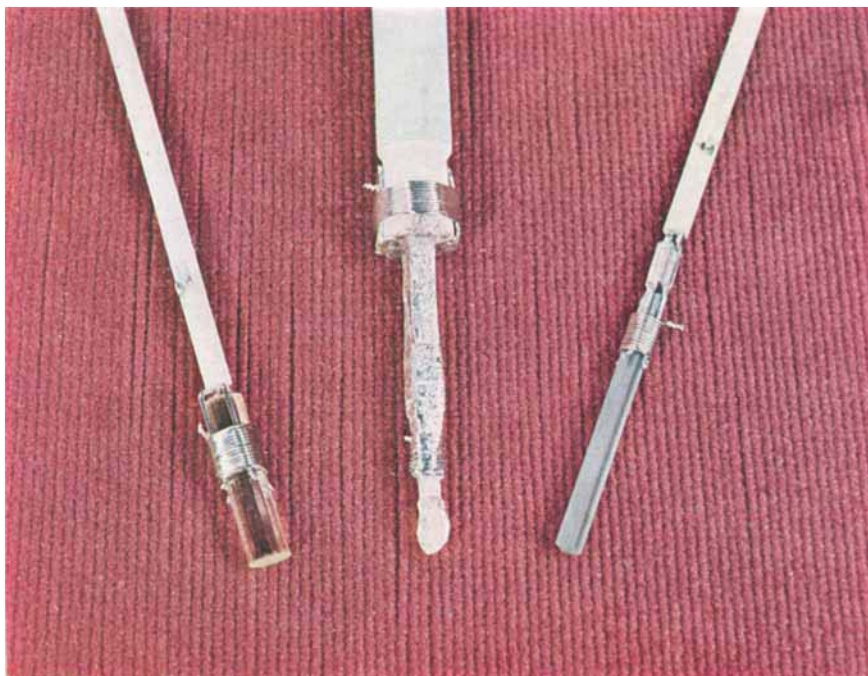
Fig. 4 Seed holders constructed from strip and wire. Their materials are selected to suit atmosphere and temperature. That on the left was made from platinum and was used for Ba_xSr_{1-x}Nb_2O_6 , that in the centre was for melts giving off corrosive vapours and that on the right in 40 per cent rhodium-platinum was for Y_3Al_5O_{12}
