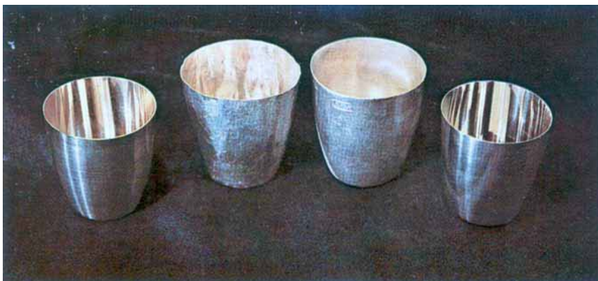
Fig. 13 Four platinum crucibles fabricated by Johnson Matthey Metals Limited. The left-hand pair was made from conventional platinum 0.25 mm thick. The used crucible was in laboratory use for three months – large grain structure and deformation caused by handling are evident. The right-hand pair was made from ZGS platinum 0.15 mm thick and weighs 40 per cent less than conventional crucibles. The used crucible was also in general laboratory use for three months but the grain structure is fine and it has retained its original shape
