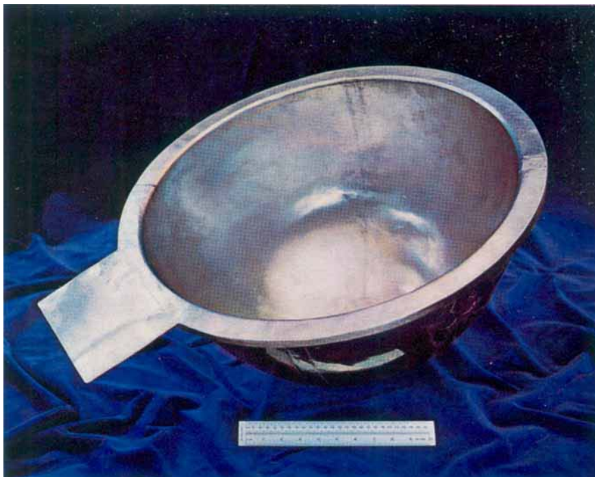
Fig. 14 A glass holding bowl approximately 50 cm diameter and 30 cm deep. Formerly made from 10 per cent rhodium-platinum sheet 0.030 inch thick, it is now made from ZGS platinum 0.025 inch thick. The use of ZGS platinum is expected to double the life of the bowl
