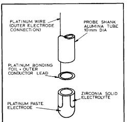
Fig. 5 Here reaction bonding is used to join an alumina tube of appropriate length to a zirconia cup. This is platinised on both the inner and outer surfaces to form the electrodes of an oxygen sensor. The outer electrode is connected by the platinum foil bond to a platinum wire and hence to the terminal head
