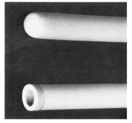
Fig. 4 Compared with a conventional domed end ceramic sheath (top), the sheath with a platinum foil window (bottom) permits a more rapid response to temperature change
