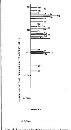
Fig. 2 Superconducting transition temperatures, plotted here on a logarithmic scale, show that the transition in rhodium occurs approximately three orders of magnitude below those of iridium and ruthenium
