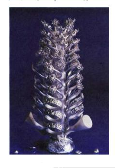
two alloys are recommended, 4.5 per cent cobalt-platinum with an as-cast hardness of 135 Hv, and where a soft alloy is required 4.5 per cent palladium-platinum (as-cast Hv = 65).
