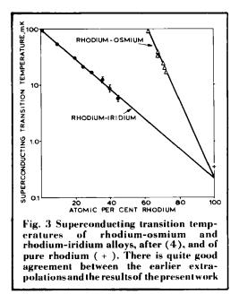
superconductive transition temperatures, shown in Figure 2, the transition in rhodium occurs at extremely low temperatures: the transition temperature of  $325 \ \mu K$  is approximately three orders of magnitude below those of the neighbouring elements iridium (0.1 K) and ruthenium (0.49 K).
