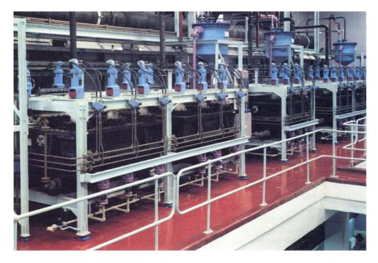
Fig. 3 After the extraction of gold, iron and tellurium, the platinum group metals are extracted. The separation of platinum, palladium and iridium relies upon a particular metal being selectively extracted from the aqueous phase by an immiscible organic solvent in counter-current mixersettler boxes
