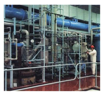
Fig. 2 In the feed preparation area the platinum group metals concentrate is dissolved in acid by reaction with chlorine gas. After any insoluble residue has been filtered off the solution is pumped to the solvent extraction area
