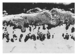
Fig. 1 This cross-section through the surface of a sample of IN792 + Hf oxidised in air for 500 hours at 1100°C shows the chromia-rich scale that exhibits poor adhesion, and a line of aluminium-rich internal oxides which is always present below the surface. Further bands of internal oxide are formed when the outer scale spalls  $\times$  700
