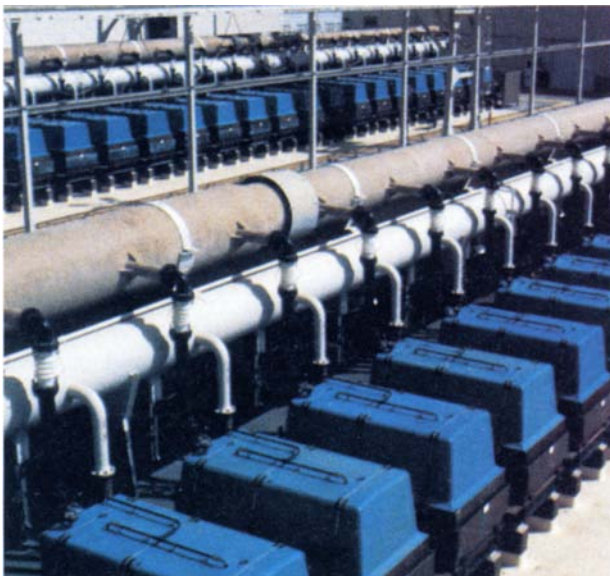
Fig. 8 View of a cell room in a chlor-alkali plant in Saudi Arabia, which uses diaphragm cell technology. Diaphragm cells produce around 75 per cent of the chlorine and caustic soda in the world Courtesy of OxyTech Systems, Inc.
