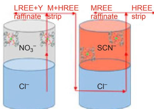
Fig. 9. General representation of the separation of REE by split-anion extraction developed by KU Leuven, Belgium. Comparison with conventional route
