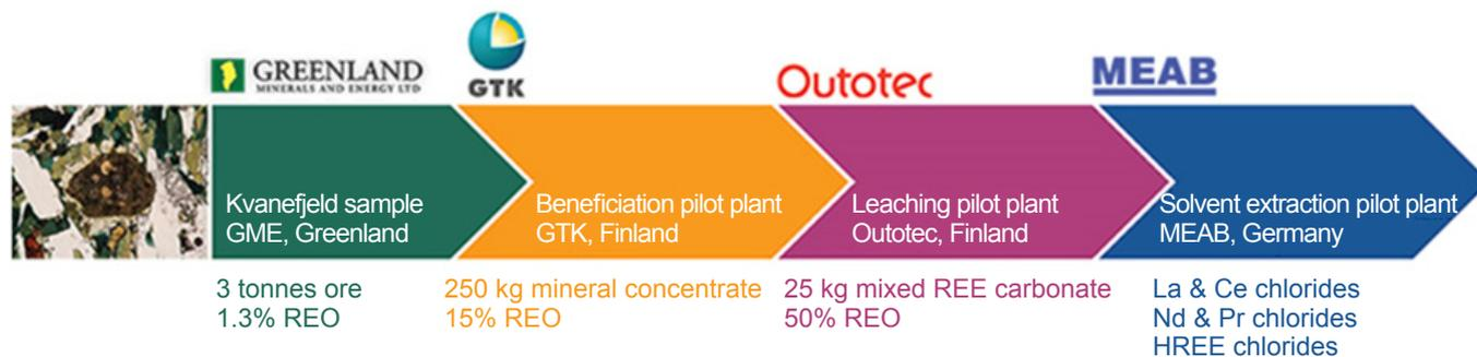
Fig. 5. Pilot achievements on the Kvanefjeld ore
