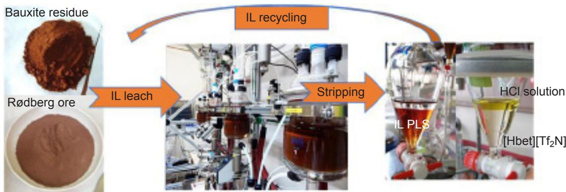
Fig. 6. Ionic liquid leaching of Rødberg ore and bauxite residue. IL = ionic liquid; PLS = pregnant leach solution. Visual flowsheet with demonstration prototype plant designed by MEAB and built in NTUA, Greece
