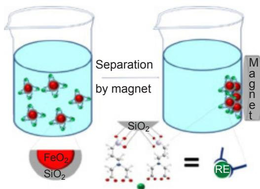
Fig. 8. Schematic presentation of hybrid magnetic adsorption of REE developed from SLU
