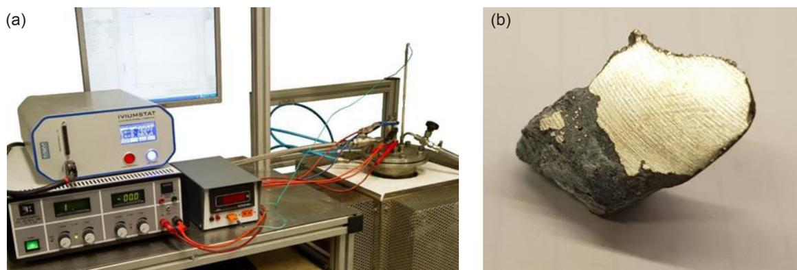
Fig. 10. (a) Optimised molten salt electrolysis cell setup; (b) didymium alloy obtained by electrodeposition in  $\text{PrF}_3\text{-NdF}_3\text{-LiF}$  electrolyte at IME Process Metallurgy and Metal Recycling laboratory of RWTH Aachen, Germany
