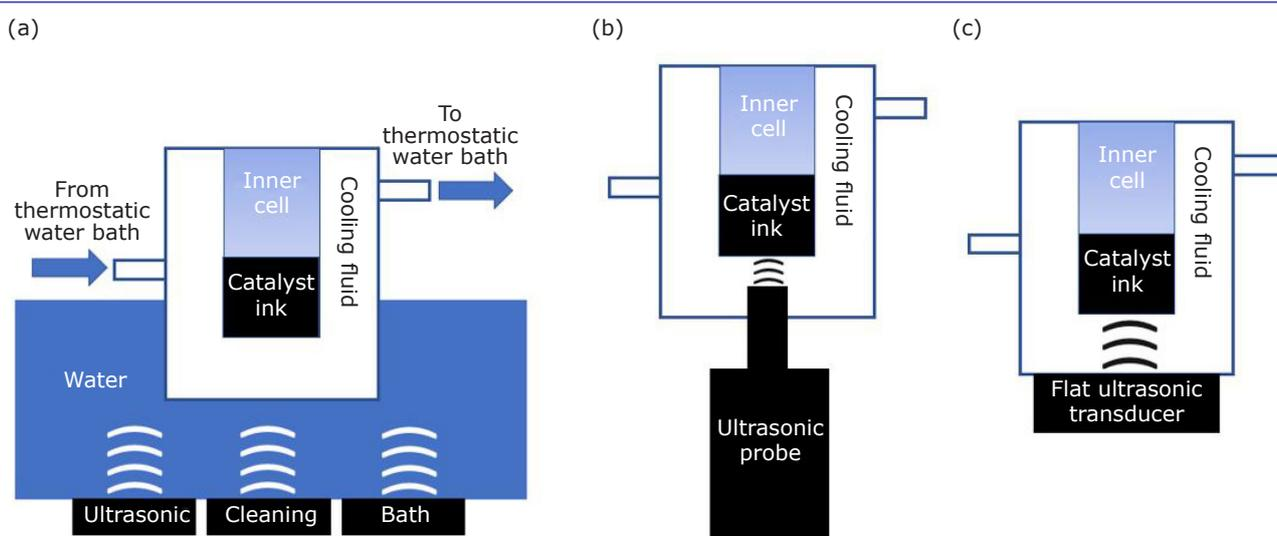
Fig. 6. (a) Thermostatically regulated reaction cell placed directly in the ultrasonic bath; (b) thermostatically regulated reaction cell with the ultrasonic probe in a 'face-on geometry'; (c) thermostatically regulated reaction cell integrated with a flat ultrasonic transducer
