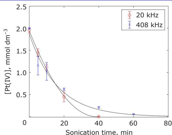
Fig. 5. Concentration of platinum(IV) in solution as a function of ultrasonication time under 20 kHz and 408 kHz. Reproduced from (37) under Creative Commons Attribution-NonCommercial 3.0 Unported (CC BY-NC 3.0)
