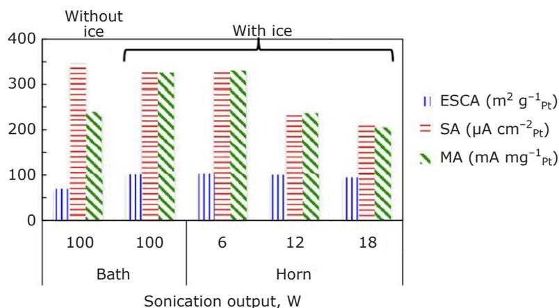
Fig. 3. Impact of cooling of catalyst ink using an ice-water bath during ultrasonication as well as ultrasonicator type and ultrasonication time on ECSA, SA and MA of platinum/high surface carbon fabricated using the Nafion<sup>®</sup>-free stationary air drying technique. Reproduced from (12) under Creative Commons Attribution 4.0 International (CC BY 4.0)
