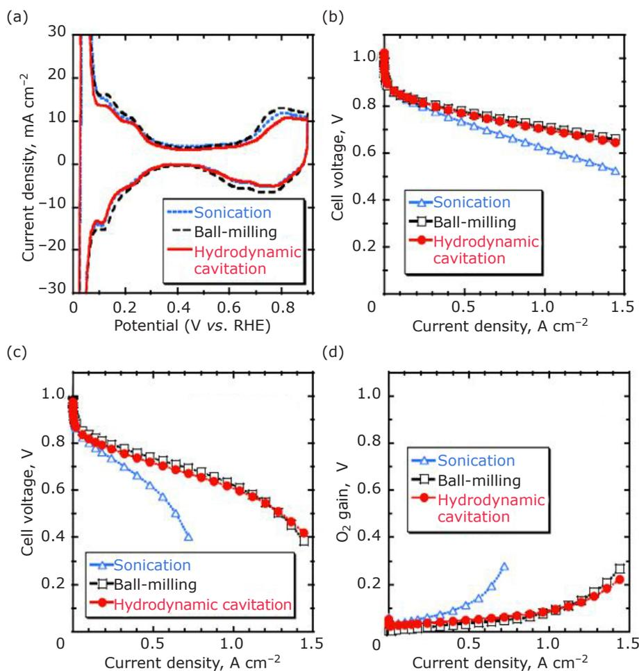
Fig. 8. (a) CV curves IV curves at 80°C for: (b) hydrogen/oxygen; and (c) hydrogen/air operation; and (d) oxygen gain for the MEAs prepared using three different dispersion treatments on the catalyst slurries. Reproduced from (6). Copyright (2019) American Chemical Society
