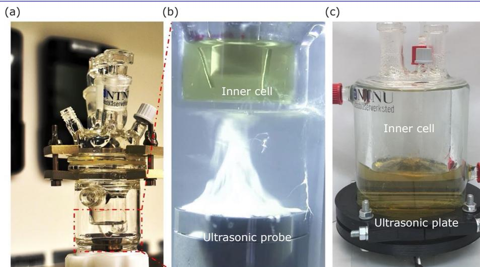
Fig. 7. (a) A double-jacketed sono-reactor with an inner cell ( $V = 10$  ml) in a 'face-on geometry'; (b) a close-up view of the ultrasonic probe (26 kHz) and inner cell; (c) a 488 kHz ultrasonic reactor with an inner cell ( $V = 100$  ml)
