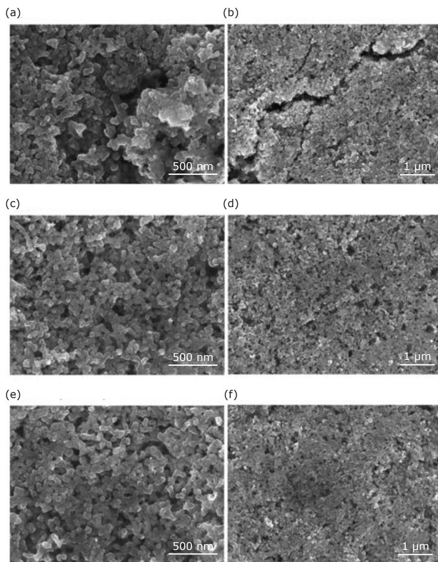
Fig. 9. SEM images of the CL on the membranes prepared using the dispersion treatments of (a) ultrasonication at 500 nm; (b) ultrasonication at 1  $\mu\text{m}$ ; (c) ball-milling at 500 nm; (d) ball-milling at 1  $\mu\text{m}$ ; (e) hydrodynamic cavitation at 500 nm and (f) hydrodynamic cavitation at 1  $\mu\text{m}$  on the catalyst slurries. Reproduced from (6). Copyright (2019) American Chemical Society
