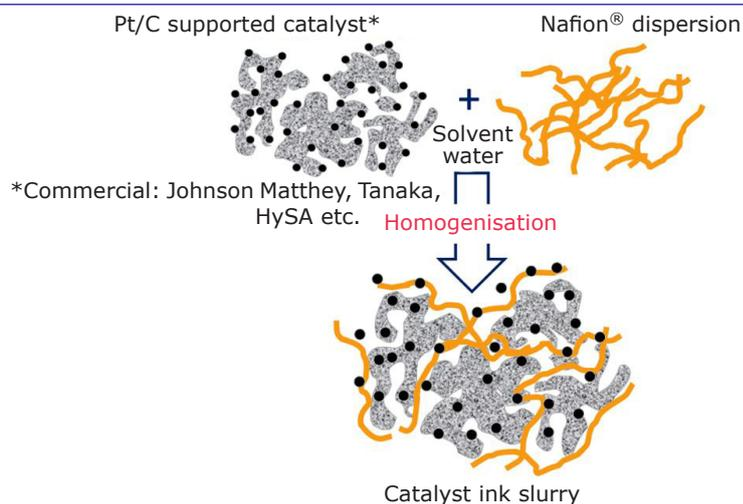
Fig. 1. Catalyst ink fabrication
