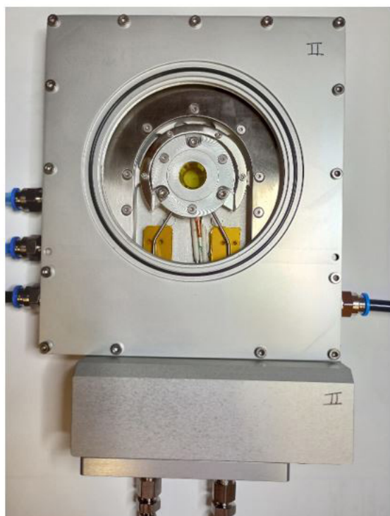
Fig. 13. Photograph of prototype in situ reaction cell used in the IR microscope in 2023 (window of the outer jacket removed). The inner heated cell contains zeolite crystals on a zinc selenide window
