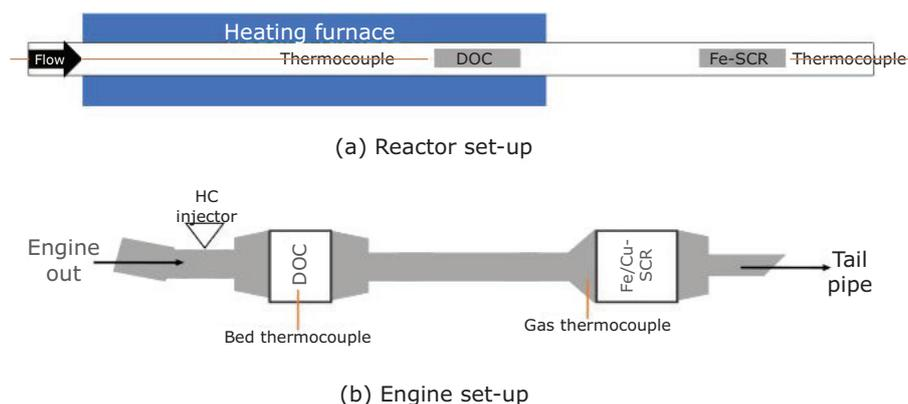
Fig. 2. Schematics of the reactor and engine setup used for platinum migration ageing
