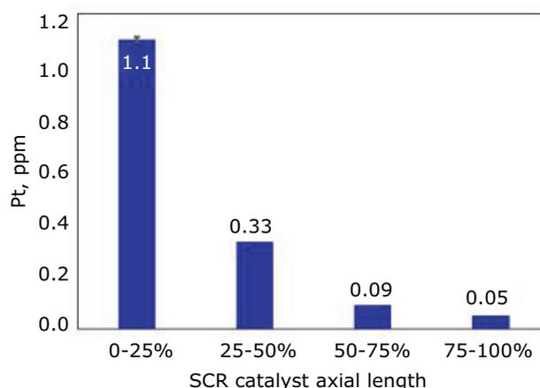
Fig. 5. Amount of platinum deposited along the 6.3" length of the zoned iron-copper-zeolite SCR catalyst during the engine ageing with the DOC-Ref exposed to 600°C for 24 h
