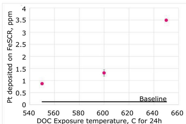
**Fig. 3.** Amount of platinum deposited on the iron-SCR catalyst during reactor ageing with DOC-Ref exposed to various temperatures for 24h. Baseline platinum level (0.1 ppm) from a fresh iron-SCR catalyst core taken from the same monolith
