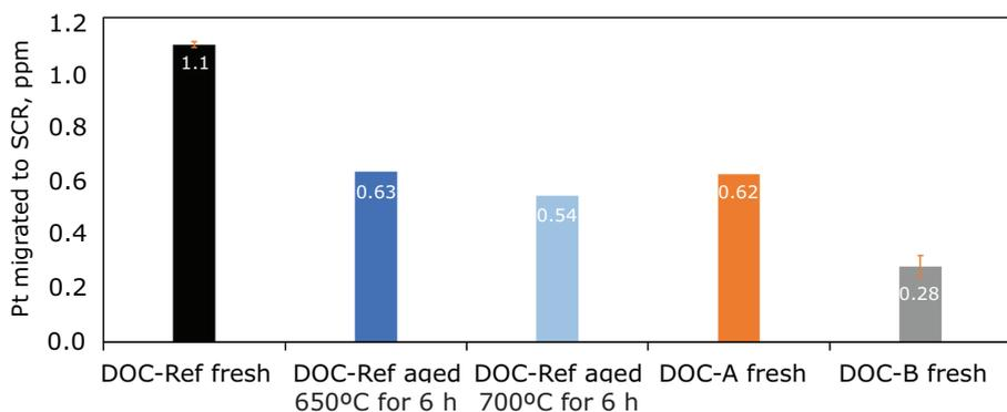
Fig. 7. Amount of platinum deposited on the zoned iron-copper-zeolite SCR catalyst inlet (1.5" length from the 6.3" long monolith) during the engine ageing with various DOCs exposed to 600°C for 24 h
