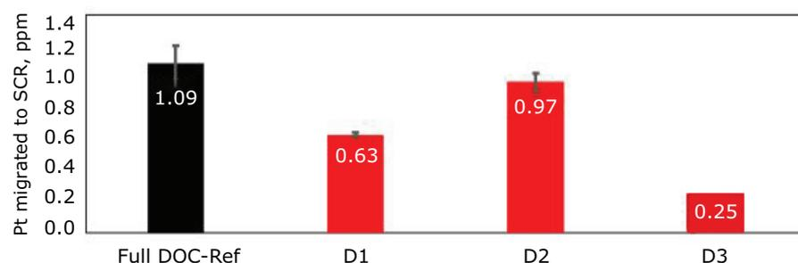
Fig. 6. Amount of platinum deposited on the iron-SCR catalyst during the reactor ageing with DOC monoliths coated only with the individual doses of the DOC-Ref (namely, D1, D2, D3). DOC exposed to 600°C for 24 h. Baseline platinum level of a fresh iron-SCR catalyst core has been removed
