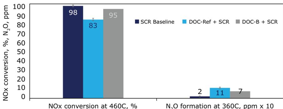
Fig. 8. NOx conversion and N<sub>2</sub>O formation of zoned iron-copper-zeolite SCR formulation during the steady state reactor testing after the platinum dioxide migration ageing on the engine with the various DOCs placed upstream
