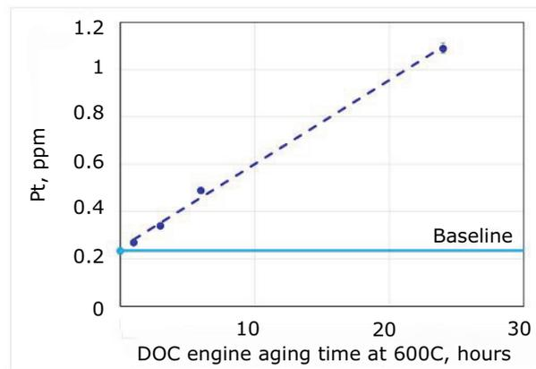
**Fig. 4.** Amount of platinum deposited on the zoned iron-copper-zeolite SCR catalyst inlet (1.5" length from the 6.3" long monolith) during the engine ageing with the DOC-Ref exposed to 600°C for different duration up to 24 h. Baseline platinum level (0.24 ppm) measured from a fresh separate SCR catalyst monolith inlet
