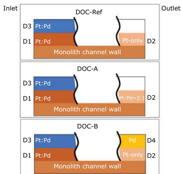
Fig. 1. DOC designs showing the inlet, outlet doses and pgm composition
