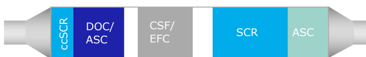
Fig. 5. Schematic of a likely example Euro 7 heavy-duty diesel catalyst system (not to scale)
