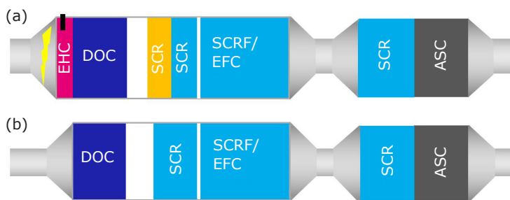
Fig. 4. Schematics of: (a) 'high technology'; and (b) likely mainstream Euro 7 light-duty diesel catalyst systems (not to scale)
