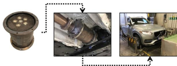
Fig. 1. Real soot collection procedure based on 10 h running aggressive RDE cycles in the vehicle chassis dynamometer. The injection timing and lambda set-point were modified to accelerate the soot collection. Reproduced from J. De Abreu Goes *et al.*, *Ind. Eng. Chem. Res.*, 2021, **60**, (47), 16899. Copyright 2021 American Chemical Society
