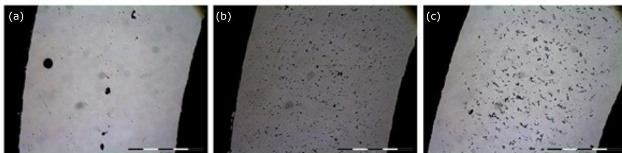
Fig. 3. Porosity in cast platinum alloys: (a) 950 platinum-cobalt; (b) 950 platinum-ruthenium; (c) 950 platinum-ruthenium-indium (35)
