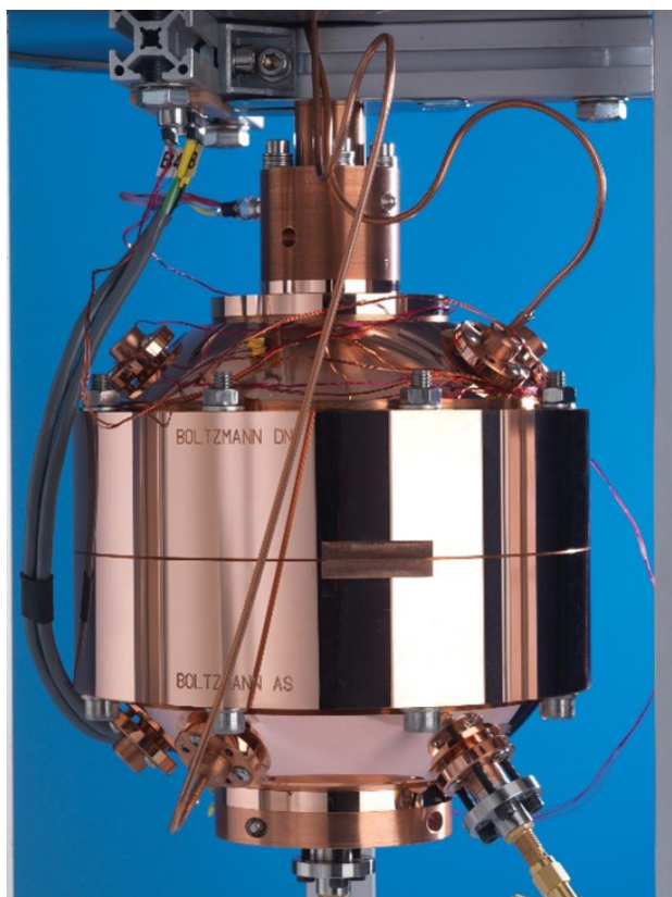
Fig. 2. The diamond turned acoustic resonator used by NPL to determine its low-uncertainty value of the Boltzmann constant
