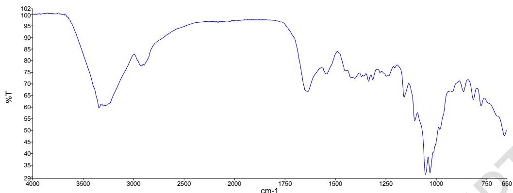
Fig 4 FT-IR spectra of BC samples treated with (a) 0.1 M NaOH; (b) 0.1 M NaOH and 1.5% (w/w) NaOCl and (c) 0.1 M NaOH and 2.5% (w/w) NaOCl.
