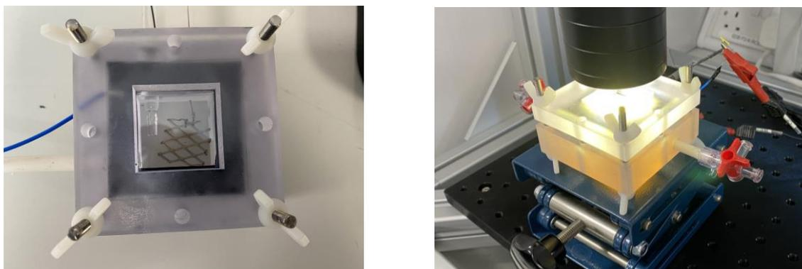
Fig. S1 – (left) Top view of the photoelectrochemical cell, using an FTO electrode; (right) photoelectrochemical cell in operation illuminated using a Pico G2V Optics solar simulator, located at 3 cm distance from the lens.
