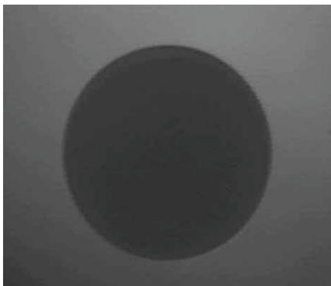
Fig. 2. Representative image of a levitated molten Os sample (~2 mm diameter)
