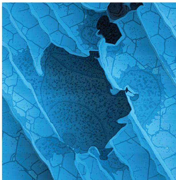
Fig. 1. Scanning Kelvin probe microscopy (SKPM) image of graphene grown on silicon carbide (SiC). Image courtesy of the National Physical Laboratory (NPL), UK
