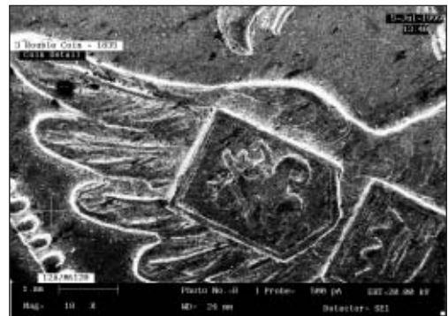
Micrographs and EDX spectra of the 3 rouble coin dated 1834; EDX: left 133 counts/s; right 15 counts/s
