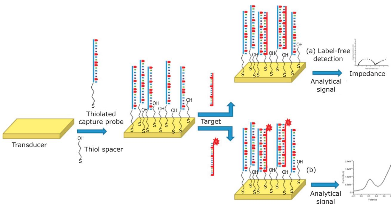
Fig. 1. Functionalisation of an electrochemical biosensor electrode for: (a) direct electrochemical gene detection; (b) labelled electrochemical gene detection. Reproduced with permission from Elsevier, copyright (2018) Elsevier
