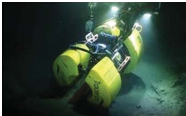
Fig. 1. The Tracerco Discovery™ tool for sub-sea pipe inspection by gamma-ray tomography (Image courtesy of Tracerco)
