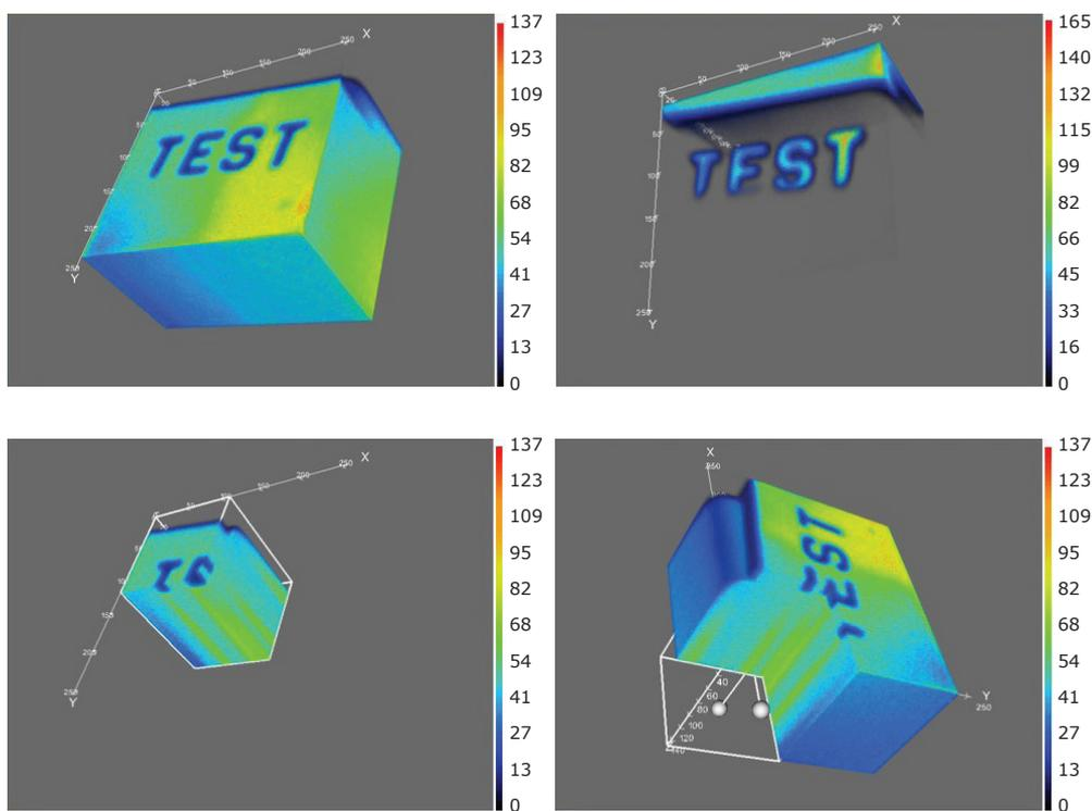
Fig. 1. SIMS images of 3D silicon/tantalum test object taken using the CAMECA SIMS instruments. Image courtesy of Mike Petty, Loughborough Surface Analysis Ltd, UK
