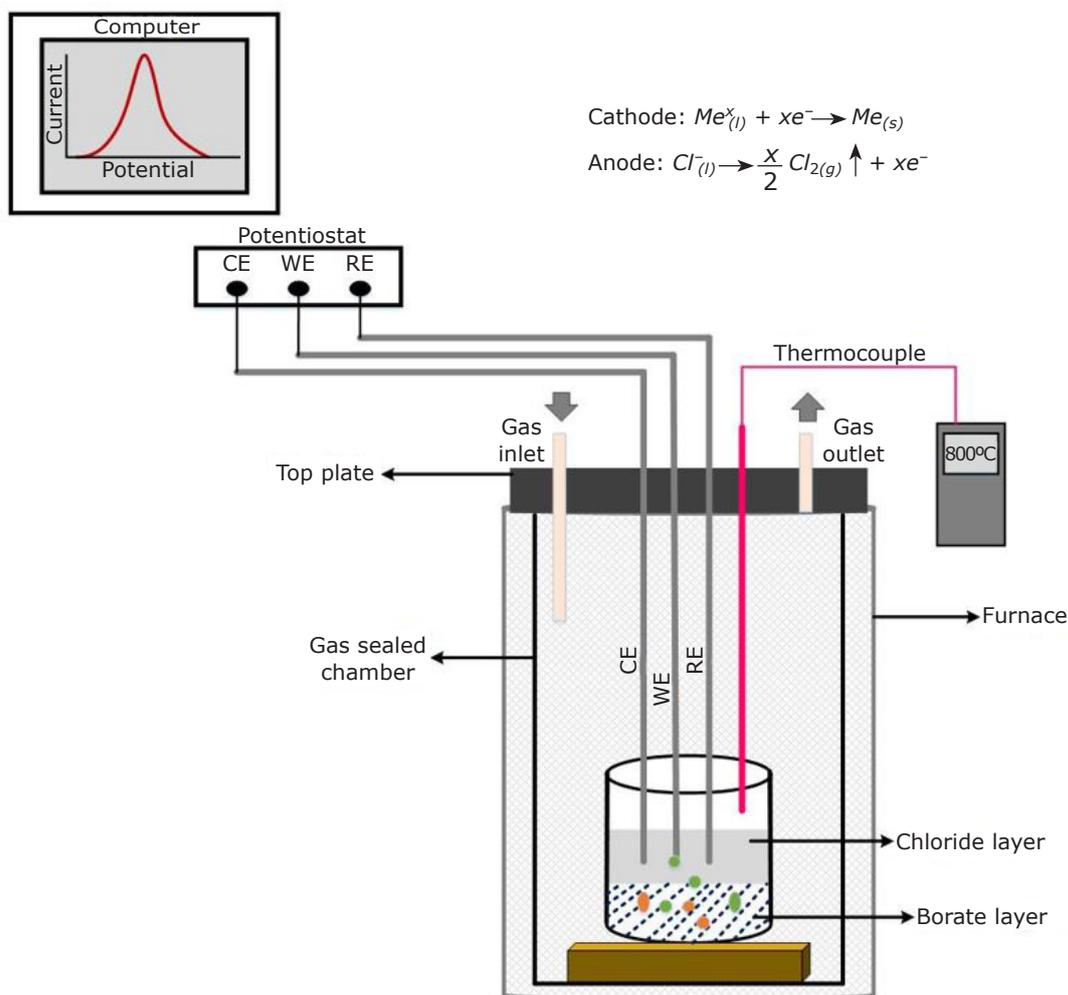
Fig. 2. Molten salt electrochemical cell scheme showing cathode and anode reactions during the process of metal deposition. Working electrode (WE) = half-cell where reaction occurs = cathode. Reference electrode (RE) = evolution of chlorine (oxidation) = anode
