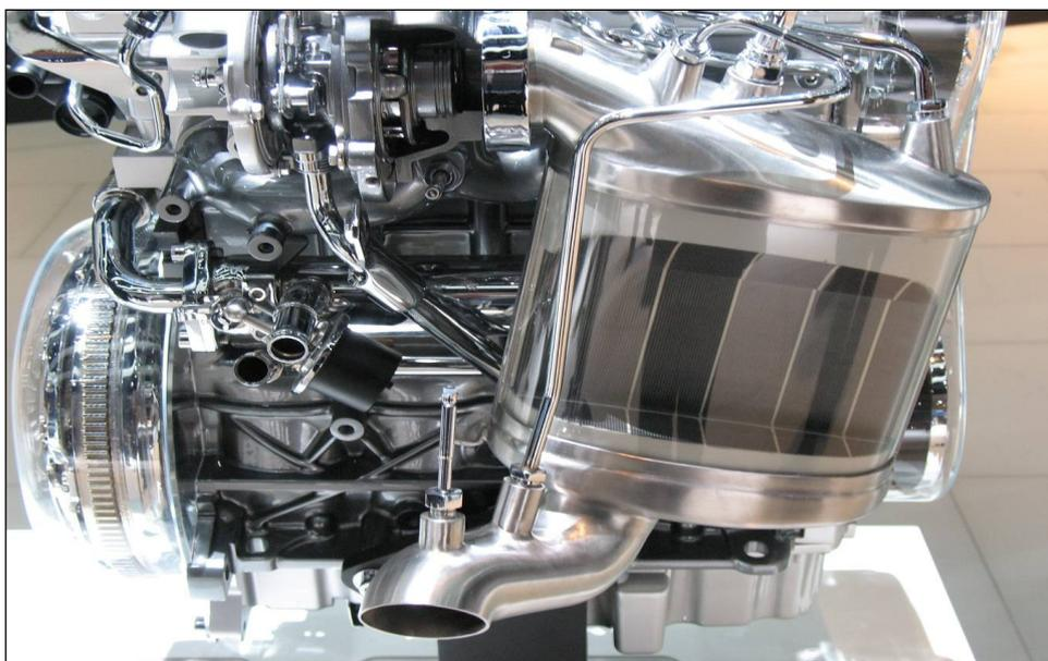
*Fig. 2. Cutaway view of a catalysed soot filter (CSF) mounted directly on the turbocharger of a passenger car diesel engine. This cost-effective technology efficiently controls hydrocarbon, carbon monoxide and particulate emissions into the environment (Image copyright Martyn V. Twigg)*
