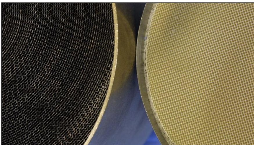
*Fig. 1. Metal foil-based substrates (left) as well as extruded cordierite substrates (right) are used to manufacture three-way catalysts for gasoline engines and oxidation catalysts for diesel engines. NO<sub>x</sub>-trapping and selective catalytic reduction catalyst formulations for lean-NO<sub>x</sub> control are also coated onto flow-through substrates*
