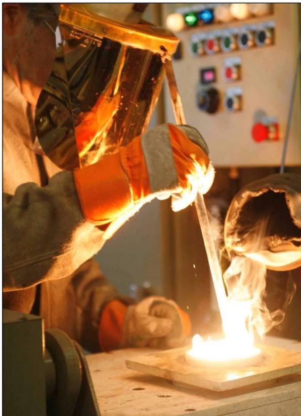
Fig. 4 Industrial casting of molten platinum.
