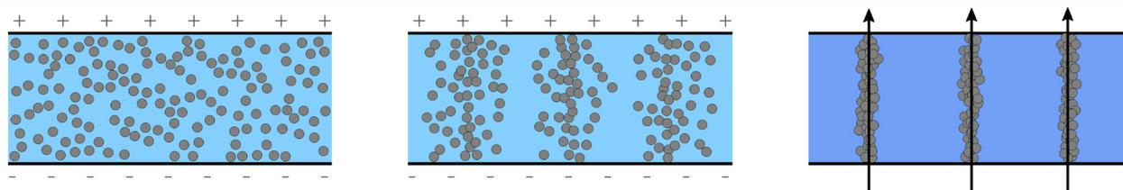
Fig. 1. Alignment of particles when exposed to an electric field in conductive films with anisotropic properties made by CondAlign, Norway (Image used with permission)
