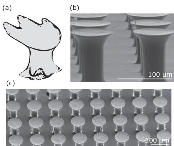
Fig. 2. (a) Shark denticle shows a divergent shape with an asymmetry in the wall-normal and streamwise directions; (b) and (c) microscopy images of the micropillar arrays, which have a similar asymmetric shape (2) Creative Commons Attribution-NonCommercial-NoDerivatives 4.0 (CC BY-NC-ND)
