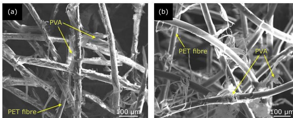
Fig. 3. SEM images show PVA linking the PET aerogel structure (4). Creative Commons Attribution 4.0 (CC BY)
