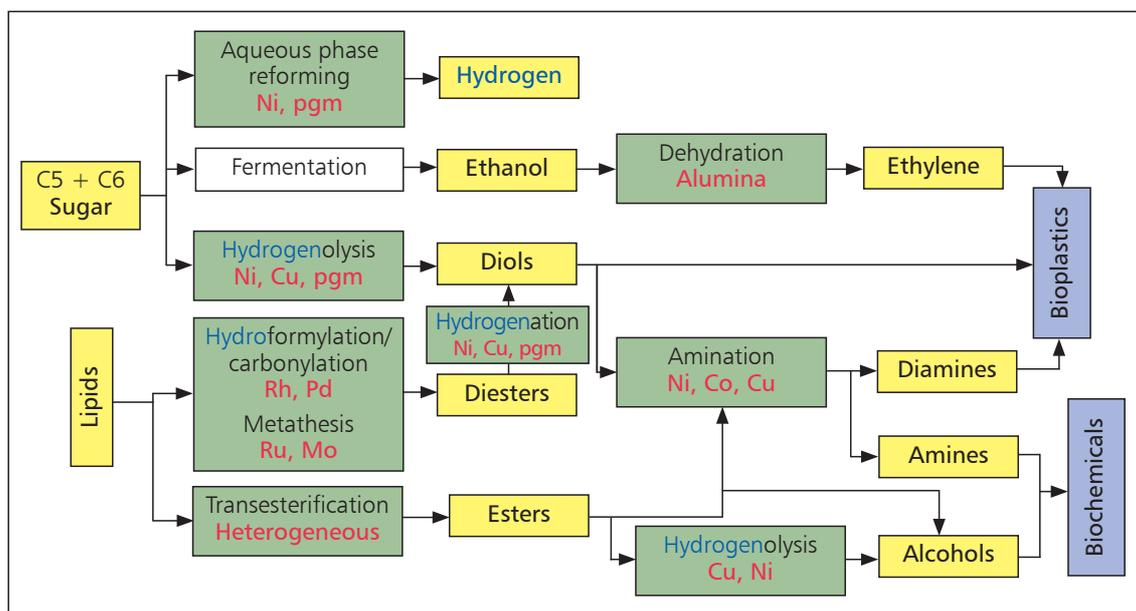
Fig. 1. Reaction scheme showing the conversion of lipids and carbohydrates to biorenewable products by a variety of pgm- and base metal-catalysed processes
