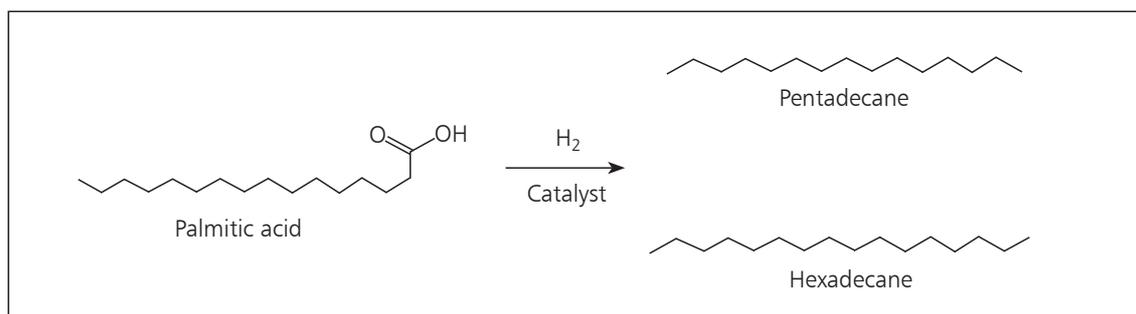
Fig. 2. The pgm-catalysed conversion of palmitic acid to long chain (C15 and C16) linear hydrocarbons such as those found in diesel fuel
