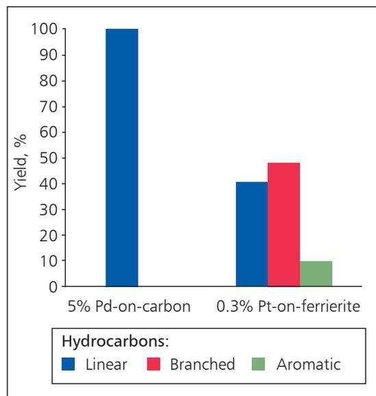
Fig. 3. Performance of palladium-on-carbon compared to a novel, bifunctional platinum-on-ferrierite catalyst for the conversion of palmitic acid to hydrocarbons
