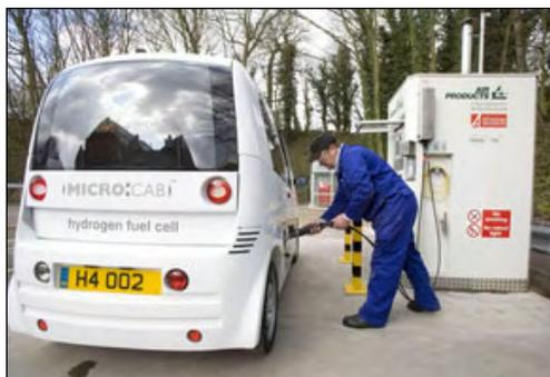
*Fig. 1 Hydrogen refuelling station and a hydrogen fuel cell vehicle at The University of Birmingham, U.K. (Courtesy of Dr Bruno G. Pollet, The University of Birmingham, U.K.)*
