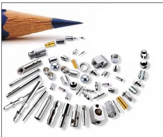
Fig. 5. Micromachined parts made from precious metal alloys for biomedical device applications, with a pencil tip for scale
