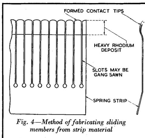
Fig. 4—Method of fabricating sliding members from strip material
