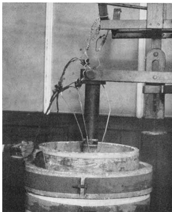
The 5 : 20 thermocouple is used in testing refractory bricks under compressive load at high temperatures in the Dorman Long research department
