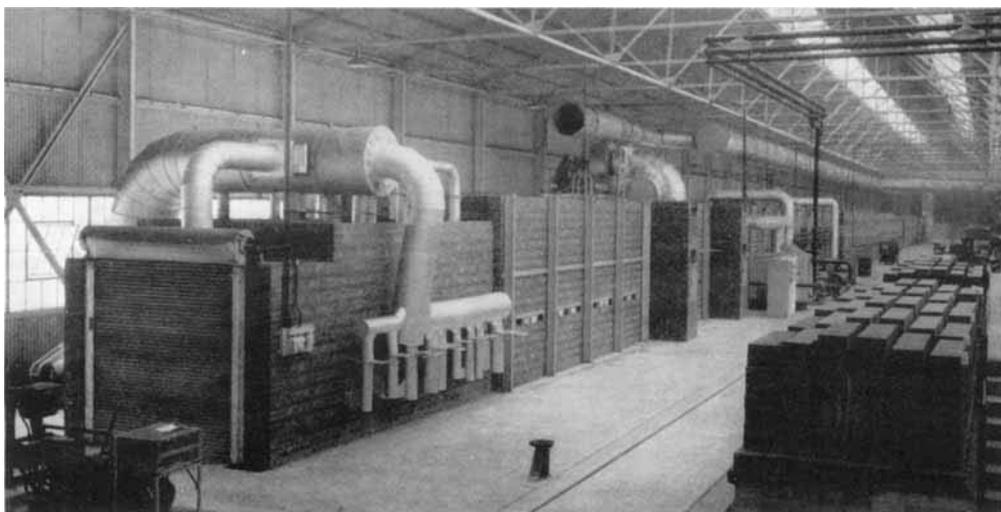
*This new tunnel kiln, firing basic refractory bricks at temperatures up to 1650° C at the Worksop plant of General Refractories Ltd., is equipped with 5 : 20 rhodium-platinum thermocouples*
