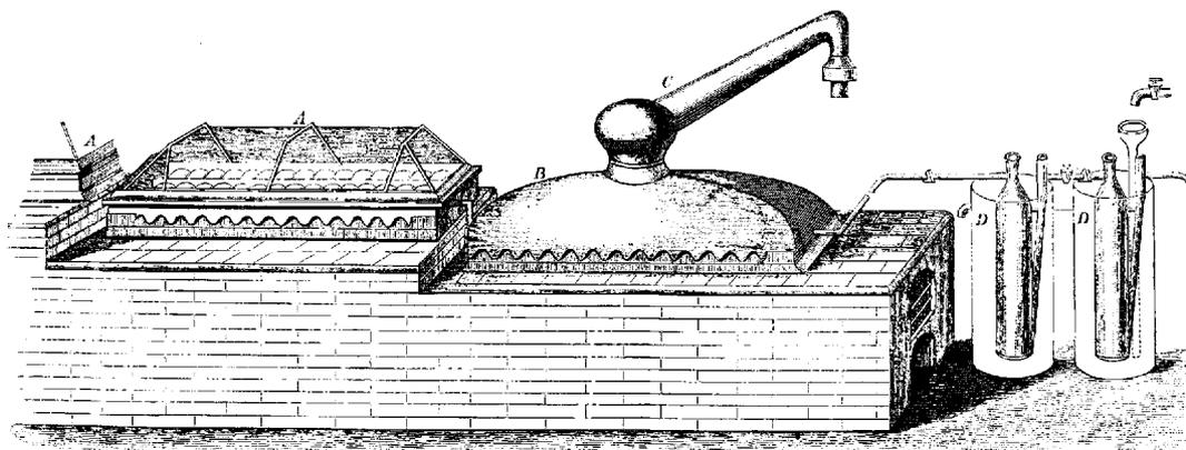
*A Delplace boiler, built by Johnson Matthey in 1876 and incorporating the corrugated bottom devised by Prentice*
