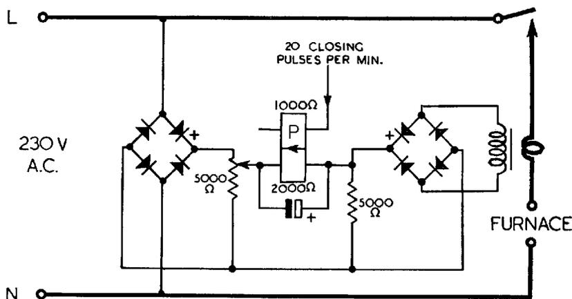
Fig. 1—Basic circuit diagram for temperature controller
