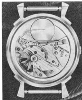
0.083 inch high, weighing only 134 milligrams each. These are heat treated, stacked in alignment, and magnetised. The new watch is said to run without attention for a year, energised by a miniature dry cell, and to keep time to an accuracy of 99.995 per cent.
