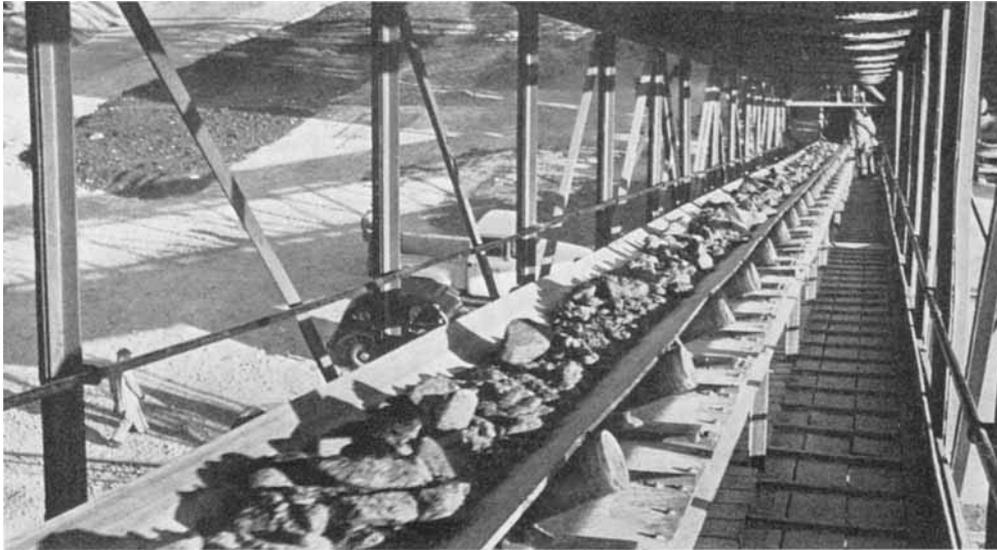
*After initial crushing the ore is transported by conveyor belt up to the sorting station in the reduction plant*
