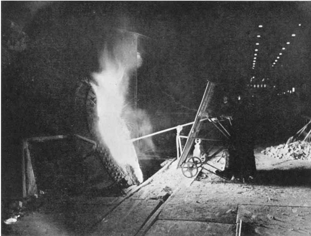
*A platinum thermocouple in use to determine the temperature of liquid steel in a Bessemer converter at the Ebbw Vale Works of Richard Thomas & Baldwins Limited*
