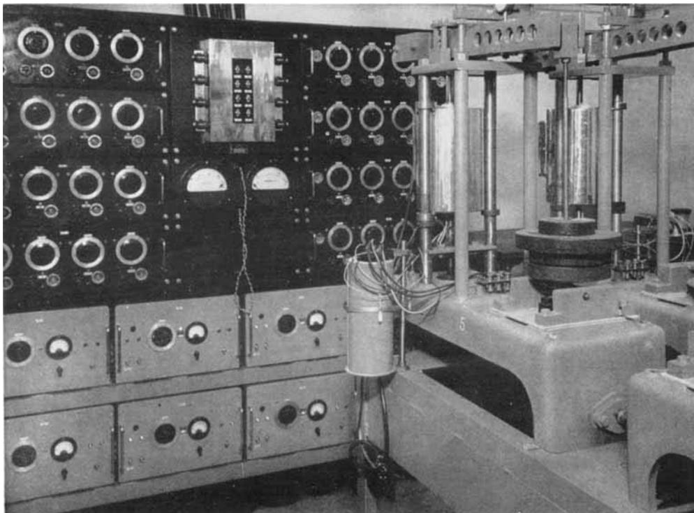
*Fig. 1—The central control panel in the creep-testing laboratory*
