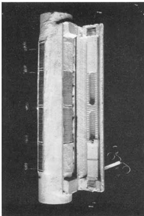
Fig. 2—A furnace unit showing the rhodium-platinum winding and the platinum resistance thermometer
