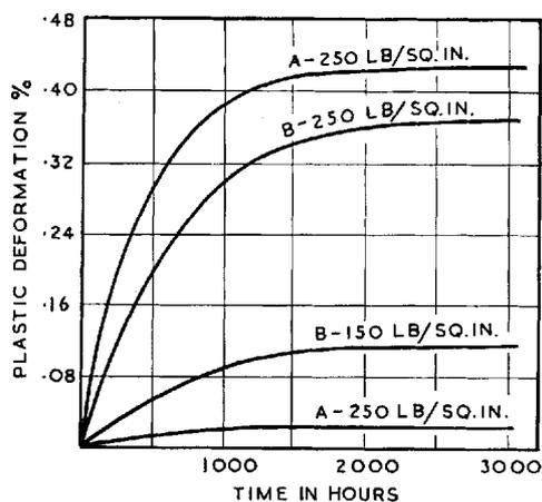
Fig. 7—Palladium creep curves at 750°C (Atkinson and Furman)
