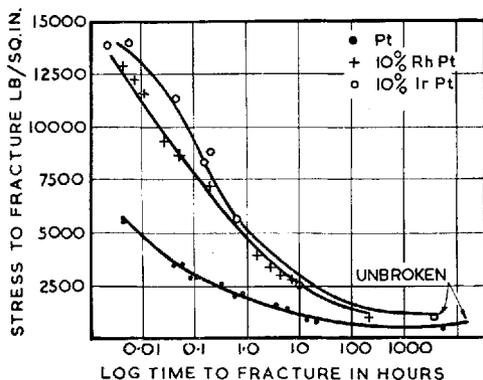
Fig. 8—Stress against log time to fracture for platinum, 10% rhodium-platinum and 10% iridium-platinum (Stauss)
