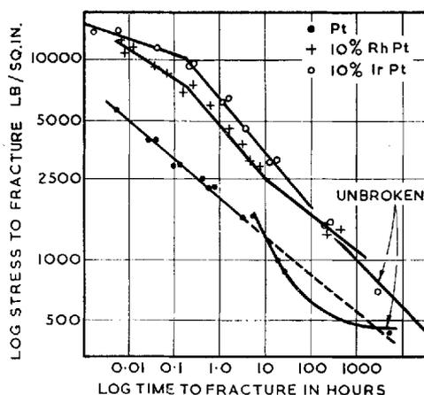
Fig. 9—Log stress against log time to fracture for platinum, 10% rhodium-platinum and 10% iridium-platinum (Stauss)
