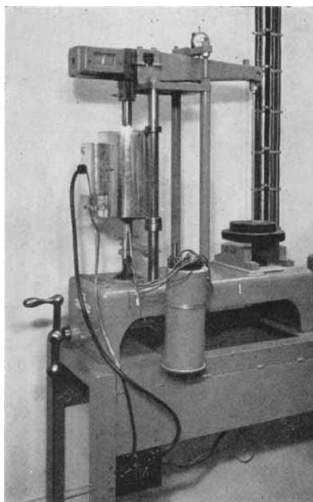
*Fig. 3—A single creep unit with a test in progress*
