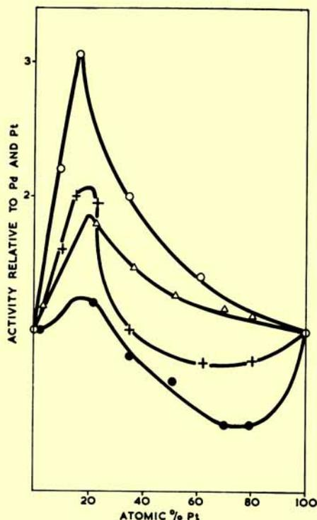
Fig. 3 The activities of reduced Pd-Pt oxides for the hydrogenation of 1-pentene in methanol (O) and for the hydrogenation of nitrobenzene in methanol (+), and of Pd-Pt alloys for propane hydrogenolysis (Δ) and for methane-deuterium exchange (●)
