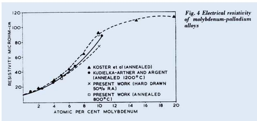
Fig. 4 Electrical resistivity of molybdenum-palladium alloys
