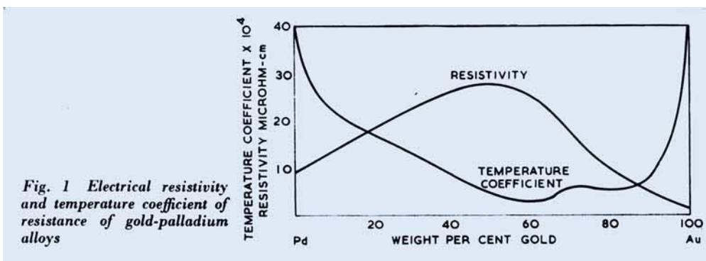
*Fig. 1 Electrical resistivity and temperature coefficient of resistance of gold-palladium alloys*
