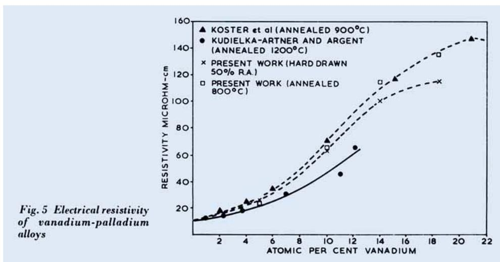
*Fig. 5 Electrical resistivity of vanadium-palladium alloys*
