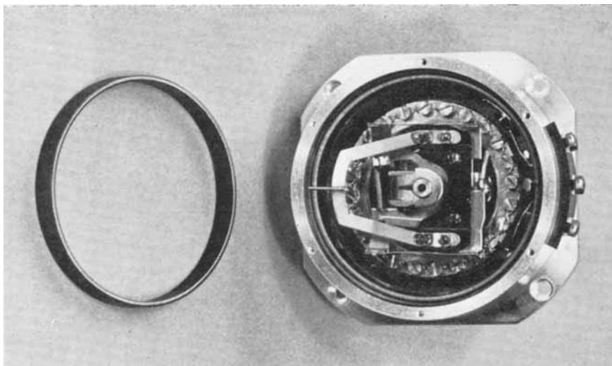
*There are many different types of potentiometers, each requiring individual selection of the winding material to meet the specified performance of the instrument. This illustration shows a Colvern cam-corrected single-turn precision potentiometer and its toroidal winding. The wire in this case is 20 per cent copper-platinum*
