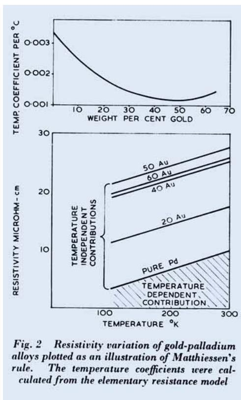
*Fig. 2 Resistivity variation of gold-palladium alloys plotted as an illustration of Matthiessen's rule. The temperature coefficients were calculated from the elementary resistance model*
