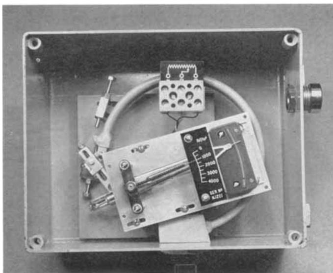
*Accurate control of temperature coefficient of resistance is essential in the manufacture of precision resistance wires. This equipment, designed and built by Johnson Matthey, gives a continuous indication of temperature and resistance of fine wires over the range  $-60^{\circ}$  to  $250^{\circ}\text{C}$*
