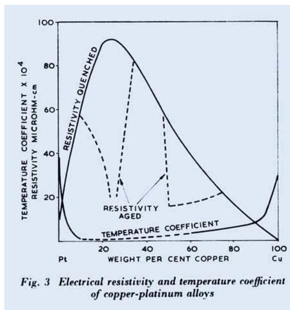
Fig. 3 Electrical resistivity and temperature coefficient of copper-platinum alloys
