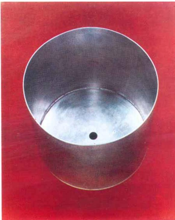
*Fig. 4 A platinum container used for the flux growth of large garnet crystals has been designed to permit draining at high temperatures*
