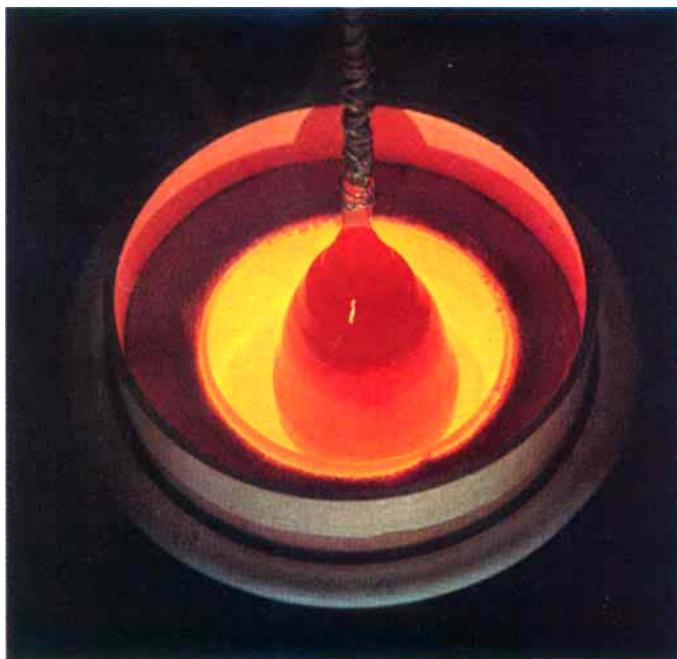
which is particularly useful for acousto-optic applications, is shown being pulled from a melt contained in a platinum crucible that is 3 inches in diameter and 3 inches high (1). The crucible is embedded in zirconia granules that are contained by a quartz liner that is closely fitted by a multi-turn r.f. coil (only the top turn is evident).
