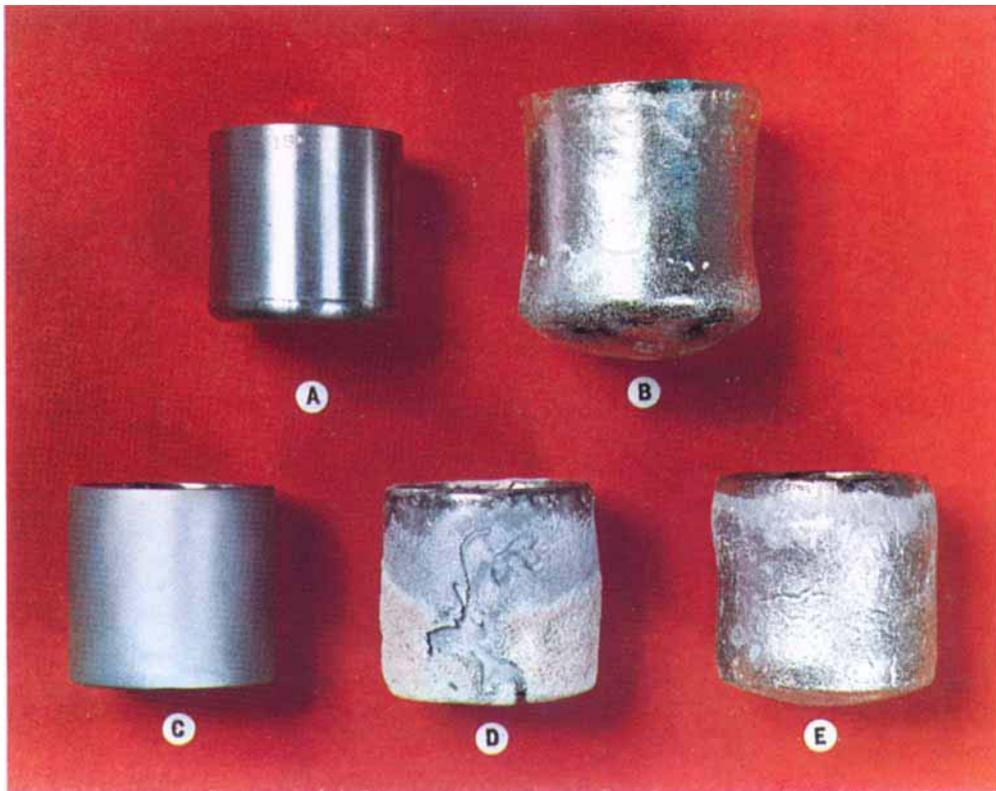
*Fig. 3 Platinum and composite platinum-iridium-platinum trilayer crucibles compared.*
