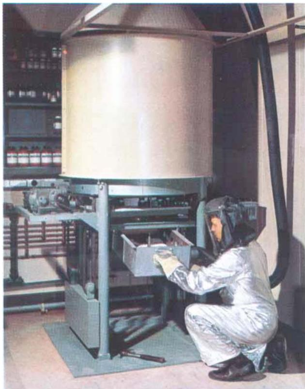
*Fig. 1 The furnace in which single crystal garnets are grown in a platinum crucible. The operator is preparing to drain off the flux by puncturing the seal in the container bottom*
