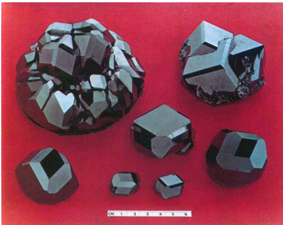
Fig. 5 Garnets grown by the technique which includes draining of the flux are used in microwave devices, delay lines, tunable lasers and bubble domain devices. Demand for them is increasing steadily
