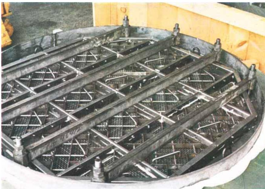
*Fig. 2 Catalyst units in Honeycat systems consist of twelve inch square and triangular modules of the platinum on Torvex catalyst. The simplicity of design aids installation of the catalyst and removal for regeneration*
