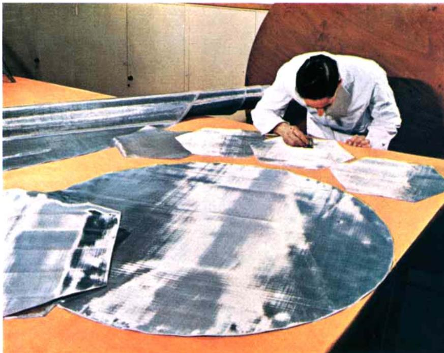
*Fig. 1 Careful inspection of gauzes fabricated by Johnson Matthey Metals before dispatch to nitric acid plants. The flat circular gauze will be installed in a medium pressure plant and the smaller hexagonal gauzes in high pressure plants. The large rolled circular gauze will be installed in a plant operating at atmospheric pressure*
