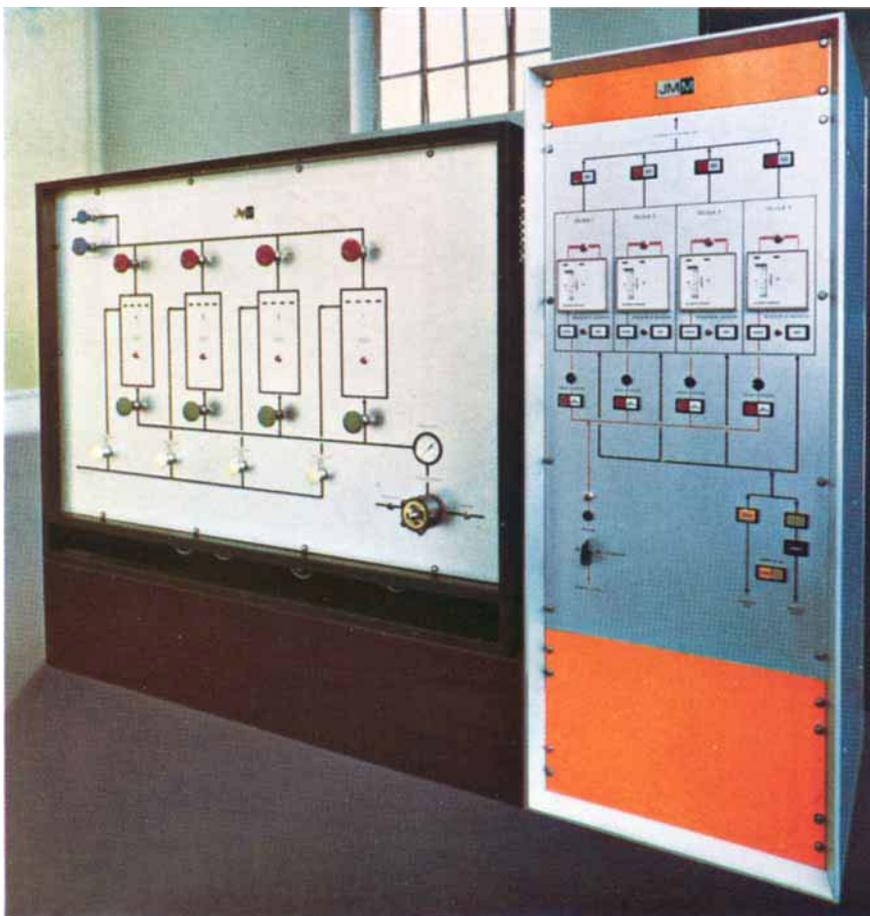
*Fig. 2 An HK 28 diffusion unit viewed from the front, showing the ergonomic layout of the controls on the pressure frame (left) and on the control console (right)*
