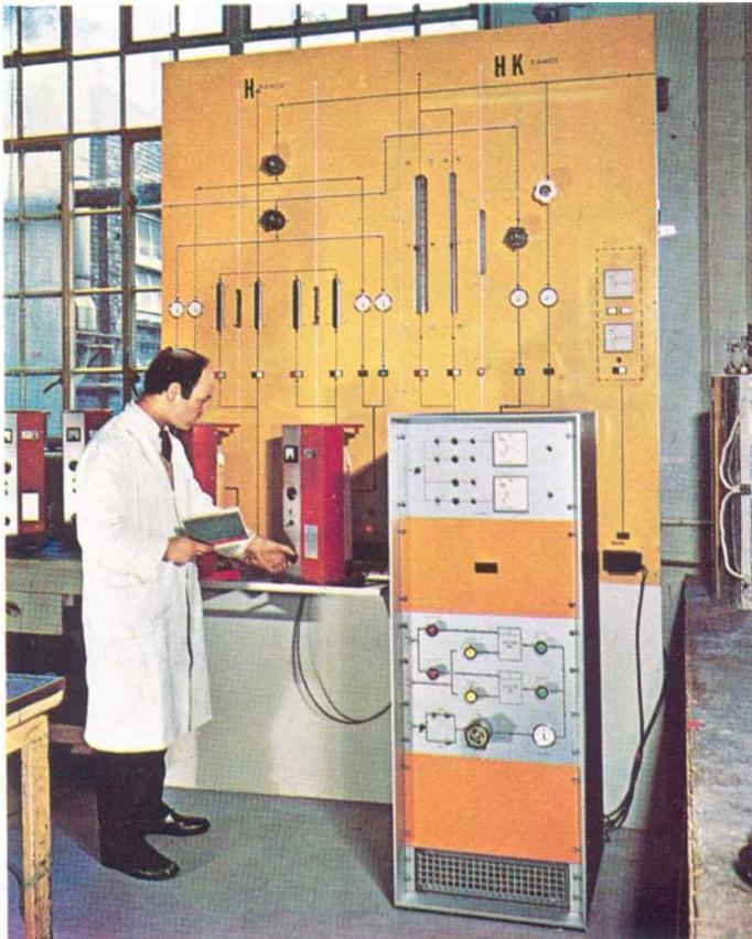
Fig. 4 Performance testing of H and HK diffusion units on a specially developed flow test rig. The operator is adjusting an H series unit while an HK series unit is on test on the right
