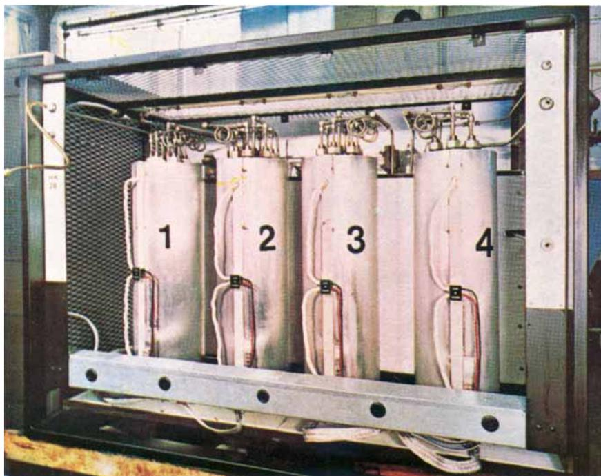
*Fig. 1 The rear of the pressure frame of an HK 28 diffusion unit, showing the compact arrangement of four diffusion modules and the ease of access for servicing*
