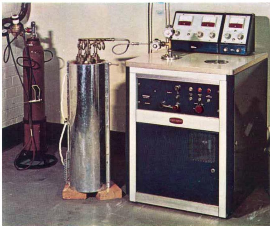
*Fig. 3 A typical diffusion module being evacuated in preparation for leak testing on the helium mass spectrometer. Only modules with leak rates less than  $2 \times 10^{-11} \text{cm}^3/\text{sec}$  at  $1 \times 10^{-5} \text{torr}$  are passed for installation in H and HK units*
