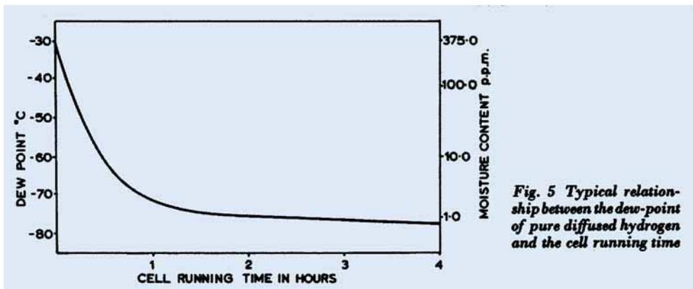
Fig. 5 Typical relationship between the dew-point of pure diffused hydrogen and the cell running time
