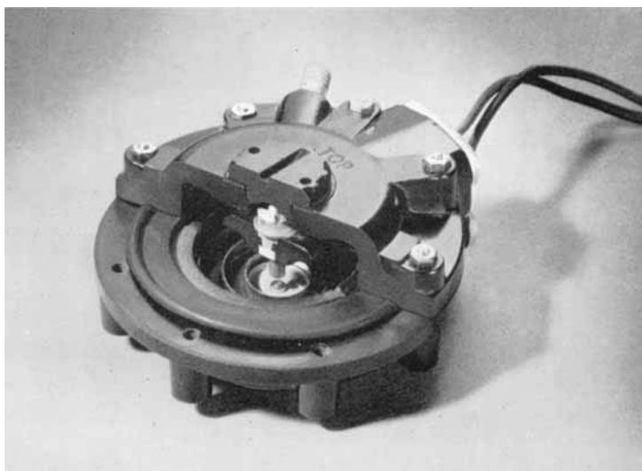
*A pneumatic contactor partly sectioned to show the contacts*
