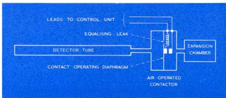
*The fundamental arrangement of the road vehicle detector. Traffic passing over and compressing the rubber detector tube gives rise to a momentary increase of pressure which operates the contacts of the pneumatic contactor*
