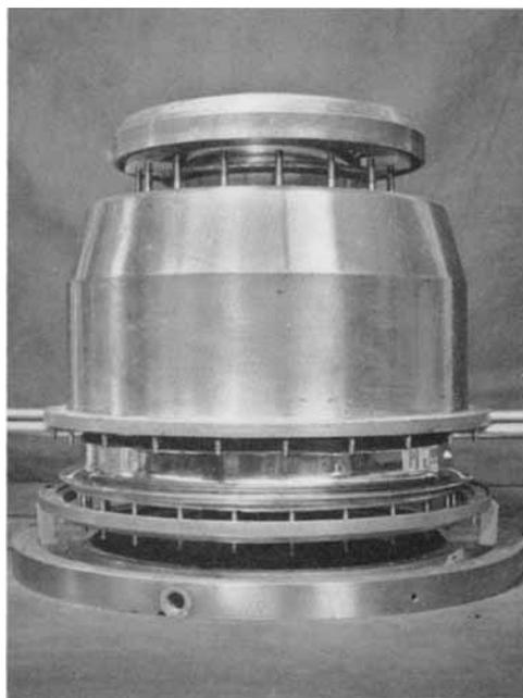
*Brush and rotor assembly of the homopolar generator*
