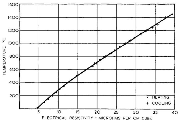
Fig. 2 Effect of temperature on the electrical resistivity of rhodium
