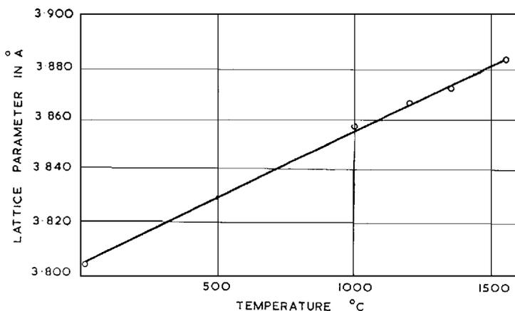
Fig. 1 Effect of temperature on the lattice parameter of rhodium
